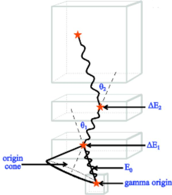
Figure 3.2: The origin cone detected by a three-stage CC. The scattering angles,  $\theta_1$  and  $\theta_2$ , as well as the initial gamma energy,  $E_0$ , can be derived from the interaction positions and the two energies deposited,  $E_1$  and  $E_2$ . The CC cannot determine the origin of the gamma ray, but because scattering angle  $\theta_1$  is known, the origin of the gamma ray is restricted to the surface of the origin cone, as described in [5].
