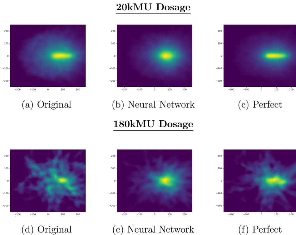
Figure 5.3: Comparison of gamma ray images reconstructed with (a/d) original data and (b/e) neural network estimation data to the (c/f) perfect reconstruction.
