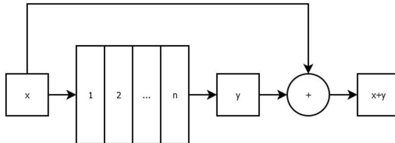
Figure 4.1: A fully connected residual block takes an input and passes it through  $n$  layers eventually adding it to the output of the  $n$  layers.
