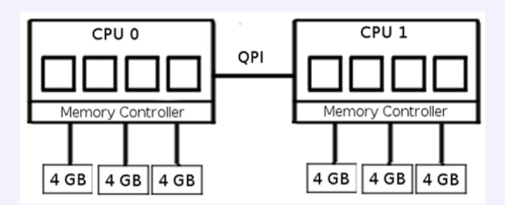
The Intel Nehalem CPUs on a compute node have 3 memory channels, each with one DIMM of 4 GB. The two CPUs are connected to each other via Intel's ultra-fast QuickPath Interconnect (QPI).
