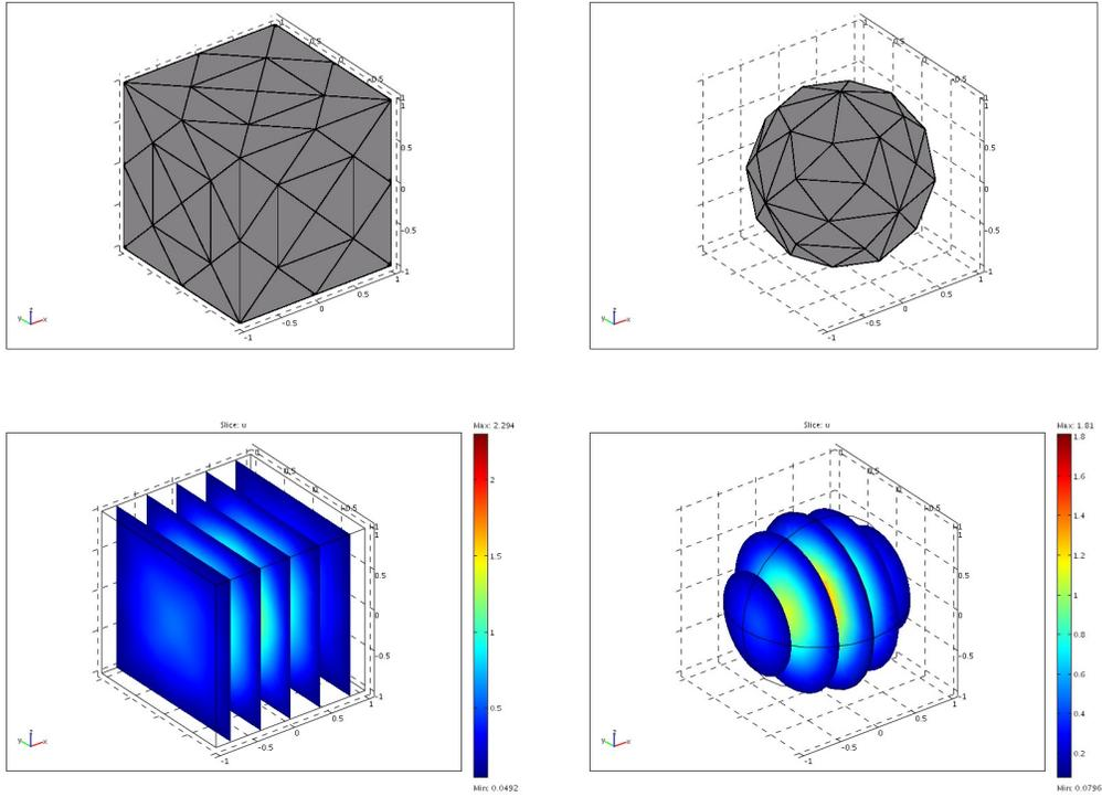
Figure 4: Mesh and solution plot for 3D polygonal (left) and non-polygonal (right) domains, non-smooth case.
