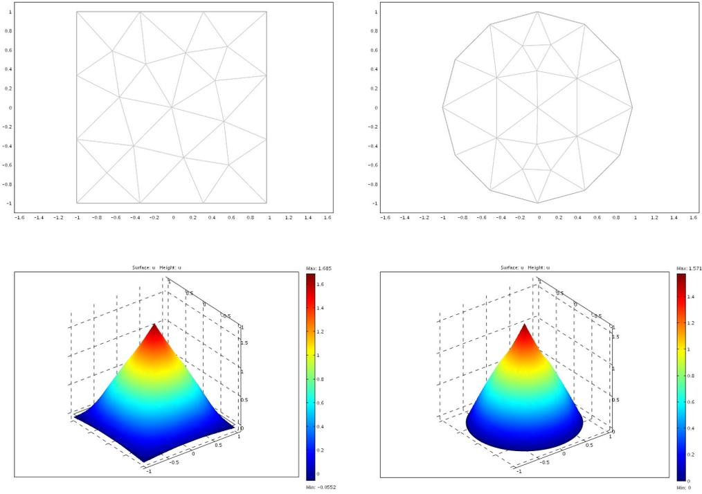
Figure 3: Mesh and solution for 2D polygonal (left) and non-polygonal (right) domains, non-smooth case.
