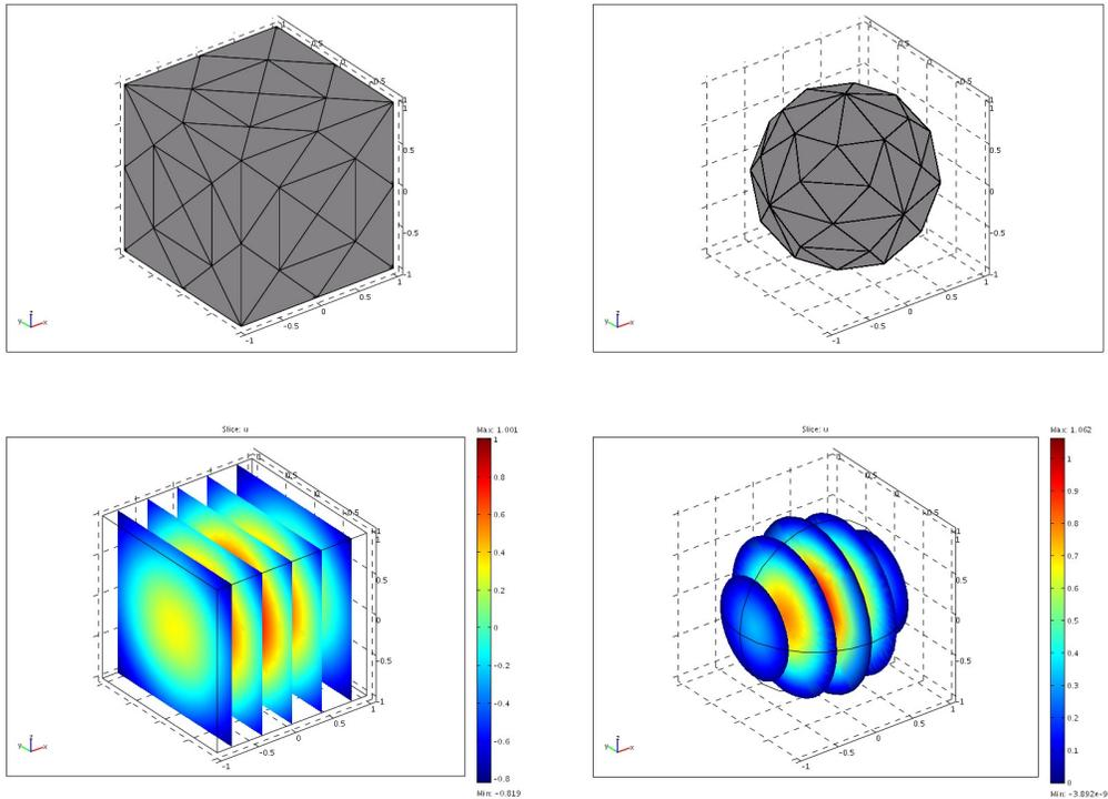
Figure 2: Mesh and solution plot for 3D polygonal (left) and non-polygonal (right) domains, smooth case.
