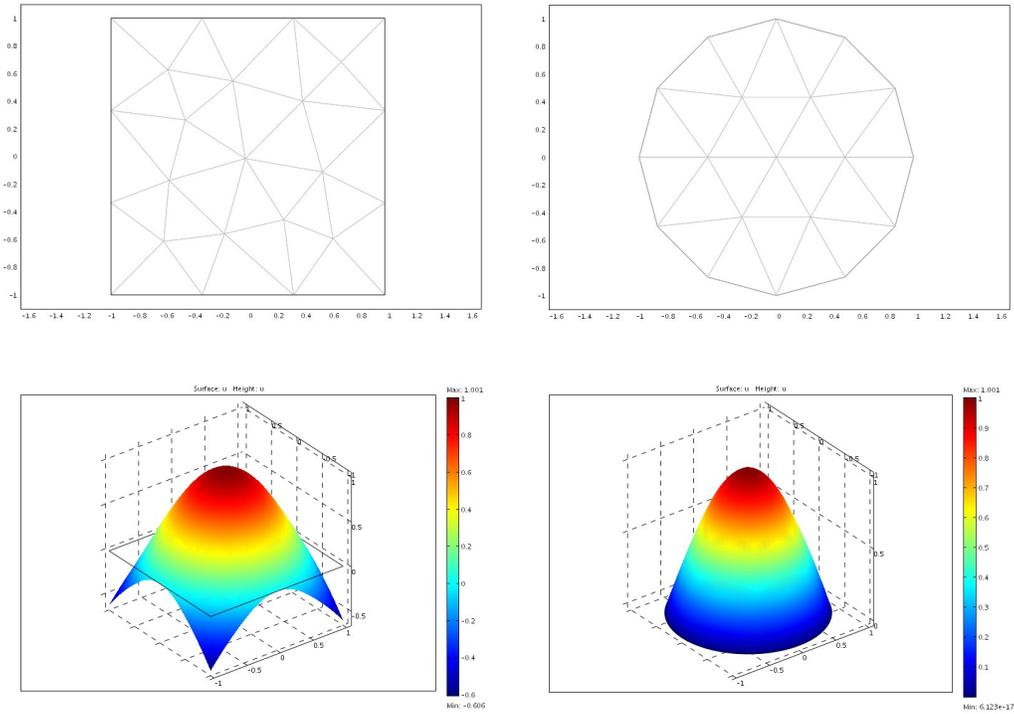
Figure 1: Mesh and solution plot for 2D polygonal (left) and non-polygonal (right) domains, smooth case.
