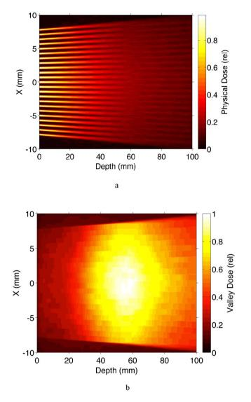
**Figure 6.** Monte Carlo simulations showing the top view of (**a**) the overall physical absorbed dose, and (**b**) the valley dose, produced in water by an array of 0.3 mm beams spaced 1 mm on center in 10-cm water.
