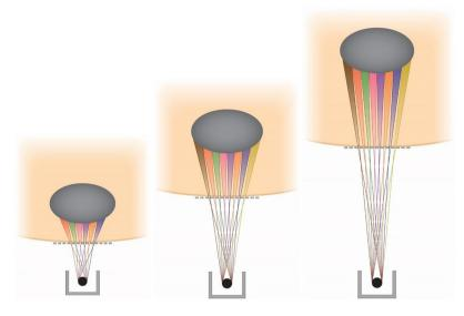
**Figure 1.** Schematic view of the method Orthovoltage x-ray minibeams (OXM). The figure also demonstrates the method of adjusting the tissue depth at which the minibeams merge by varying the distance between the source and the multislit collimator.
