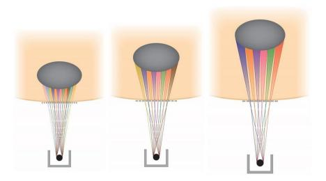
Figure 12. Adjusting the tissue depth at which the minibeams merge by varying the spacing between the minibeams.
