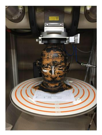
**Figure 3.** Alderson phantom positioned underneath the beam-defining collimator of the 250 kVp x-ray machine at PXI. The multislit collimator, which was used to produce Fig. 4, was positioned on the top of the phantom, and the distance between the source and that collimator was adjusted to be 295 mm.
