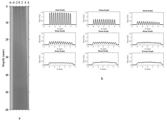
**Figure 5.** (a) Exposure of a chromographic film to an array of 0.3-mm 320-kVp x-ray minibeams spaced 1.0 mm on-center. The merging point is 3.1 cm from the collimator. (b) Lateral profiles of the film image of (a), made for nine depth points ranging from 0 mm (entrance to the film) to 80 mm, which is beyond the merging point of the arrays, which is at about 31 mm.
