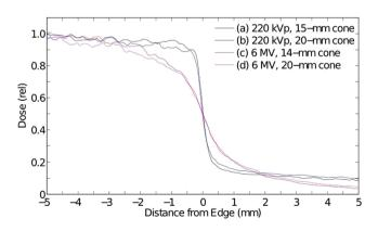
**Figure 7.** Lateral dose profiles of a 220-kVp and a 6-MV beam measured on a film stacked between two 4-cm plastic plates; it demonstrates the very large difference between the lateral dose-falloffs of these two beams, namely 80%-to-20% dose falloffs of ~0.4 mm and 2.2 mm, for the two beams, respectively.
