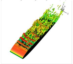
Flow field from LES of laminar-turbulent transition over a NACA0012 wing at Reynolds number 50,000. The angle of attack (AoA) is 8 degrees. Vortex structures are indicated by the Q-criterion colored with streamwise velocity.
